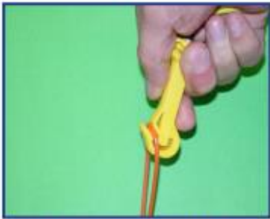
Figure 4 - Correct insertion of shock tube into EZ Connector block; one at a time.
