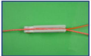
Figure 41 - Step 1, cord in center groove.
