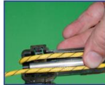
Figure 12 - Correct insertion; block open, detonating cord laid parallel to detonator and wrapped around Bunch Block.
