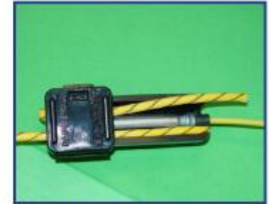
Figure 13 - Correct insertion; block closed, detonating cord laid parallel to detonator and wrapped around Bunch Block.
