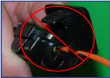
Figure 10 - Shock tube incorrectly inserted into Bunch Block; under hinge, misfire may occur.
