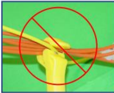
Figure 7 - Shock tube leads incorrectly seated. Yellow lead is crossed-over; mis-fire may result.
