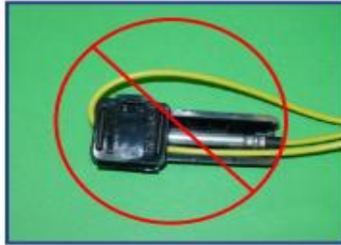
Figure 11 - Shock tube bent around nose of Bunch Block. Cut-off may result.
