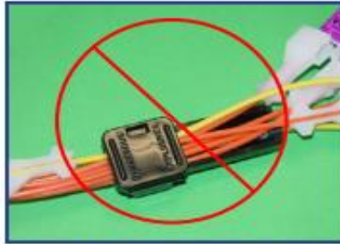
Figure 9 - Shock tube incorrectly inserted into Bunch Block; yellow lead not in direction of initiation.
