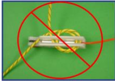
Figure 40 - Incorrect MSConnector connection. Cord not in center groove.
