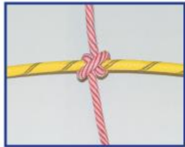
Figure 63 - Single-wrap clove hitch knot.
