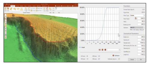
Figure 6 Software with the Kuz-Ram analysis (O-pitblast, 2019)
