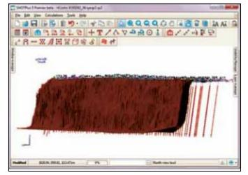
Figure 11 3D surfaces of blast field with boreholes (Shotplus 5 premier, 2019)
